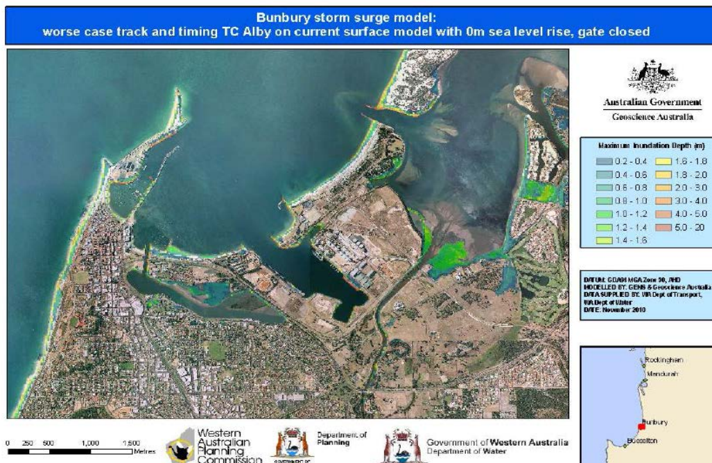
Figure 17: Inundation map for Bunbury developed by Geoscience Australia. Source: www.planning.wa.gov.au
