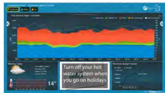
The City of Greater Geraldton investment in a 'dash-board' to continually monitor power usage at the Geraldton Aquarena.
