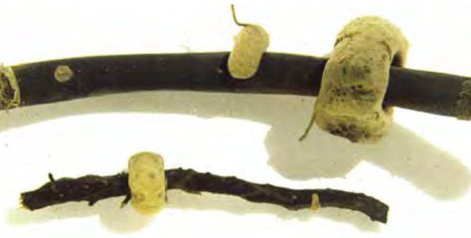
(left) Haustoria on root and telephone cable, (right) Nuytsia secateur-like cutting device
