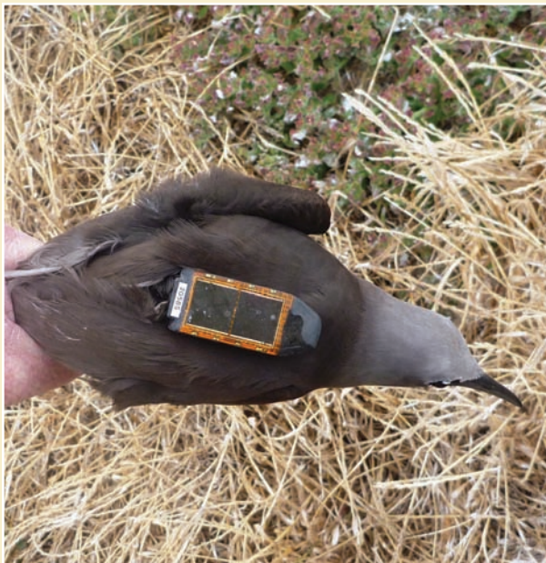
Noddy 2058 recaptured at the nest for tag removal 24 days later having made 14 foraging trips and flown 1261km.
