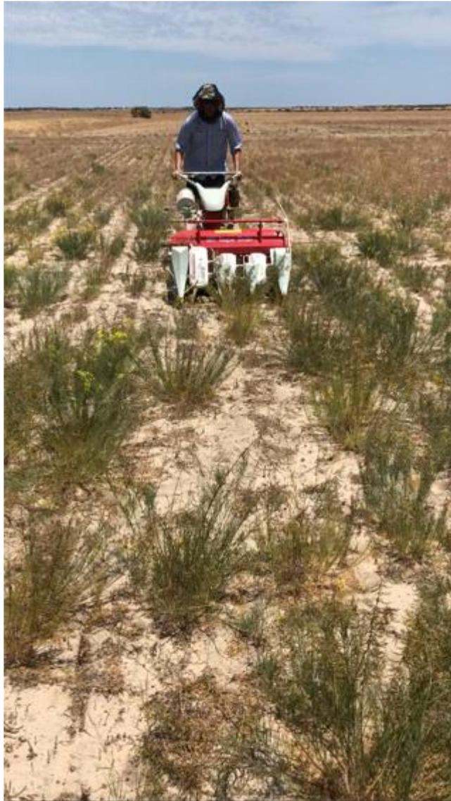
Figure 7. Harvesting Lebeckia pods with the binder / reaper machine at Binnu in November 2017.
